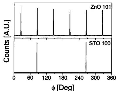
FIG. 1.  $\phi$  scans of the ZnO101 and STO 100 reflections: ZnO grows with the side of the hexagon parallel to the short side of the rectangular surface cell of STO 110.
