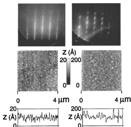
FIG. 2. RHEED and AFM images of ZnO thin films grown at 570 °C (left) and 800 °C (right); The rms roughness of the two films are 0.43 and 2.9 nm, respectively. By lowering the deposition temperature a quasi-two-dimensional growth mode can be achieved.
