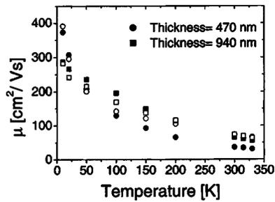
FIG. 3. Mobility as a function of the temperature for 470 and 940-nm-thick films grown by a two-step deposition. The relaxation layers are 70- and 140-nm-thick, respectively. Hall mobility (closed symbols) and mobility estimated from magnetoresistivity data (open symbols) show an exponential decay with the temperature.
